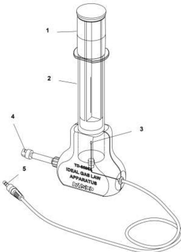
**Figure 3: A schematic of the Ideal Gas Law Apparatus. The labeled components are given below.**
