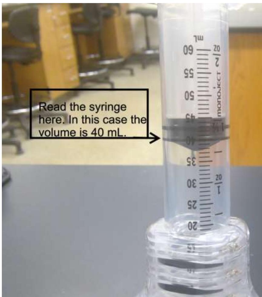
**Figure 4: How to read a syringe. Make sure you don't read the very bottom. Otherwise, all of your measurements will be much too small.**
